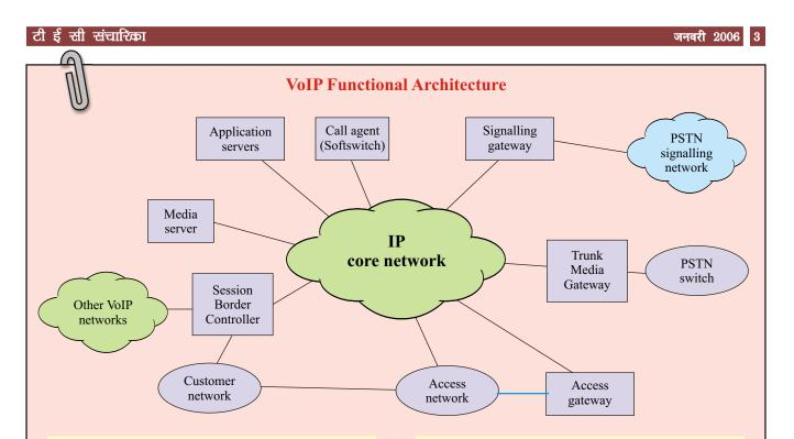
Access network (AN): The access network provides connectivity between the customer premises equipment and the access gateways in the service provider's network. There are various access methods: TDM direct access, switched TDM, broadband access (cable, DSL), IP managed Internet service, etc.
